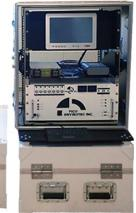
33.6 litres volume GAMMARAY SYSTEM installed in one of our aircraft.
